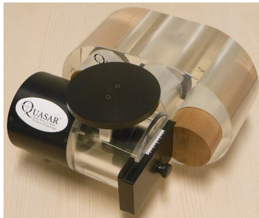
FIG. 1. QUASAR respiratory motion phantom.
