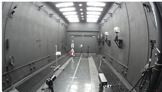
Figure 2. Spectral transmission measurement devices in the fog chamber.
