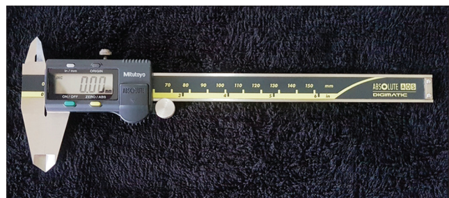
Figure 1: Digital caliper for recording measurements
