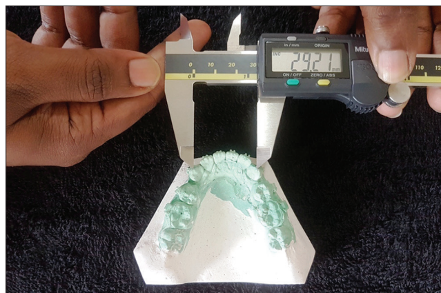
Figure 2: Measuring intercanine width
