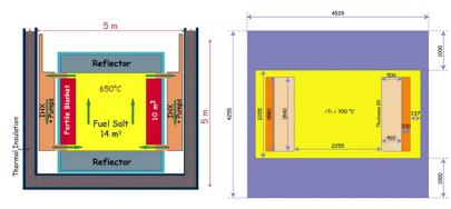
Fig 1. Geometry of the model reactor used in this study.
