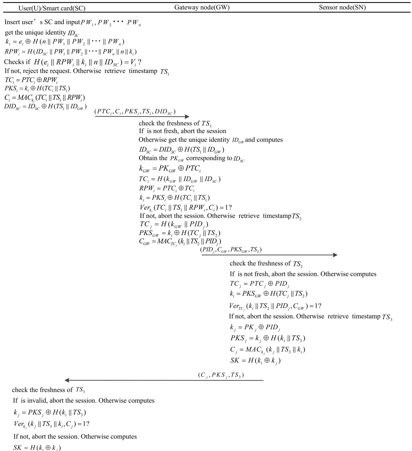
Fig 3. The login, authentication and key exchange phase of our scheme.
