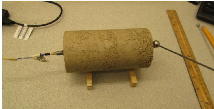
Figure 1. Cylindrical specimen and configuration for testing the longitudinal resonance frequency.
