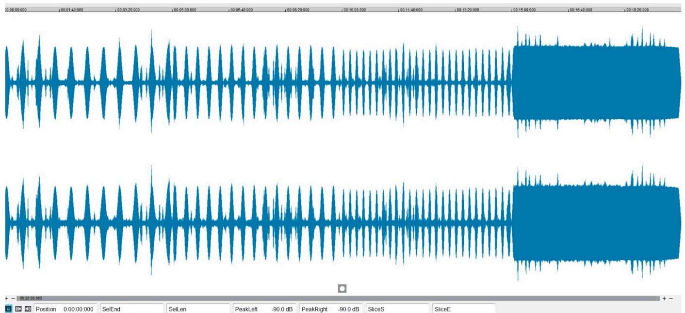
Figure A1. Visualisation of Amplitude Modulation used by Vibrobed.
