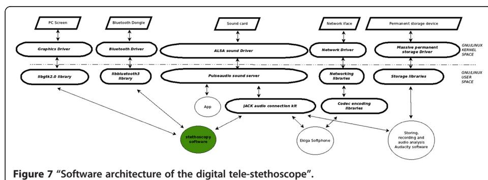
**Figure 7** "Software architecture of the digital tele-stethoscope".
