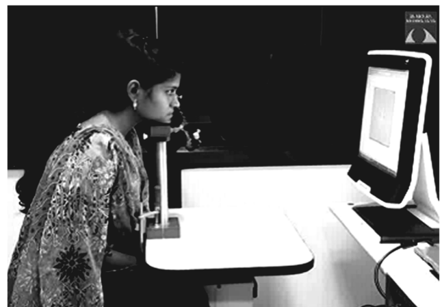
Fig. 2 The Eye Movement Perimetry (EMP) test set up consisting of eye tracking device and Thin Film Transistor (TFT) monitor
