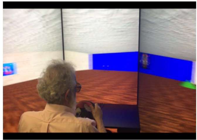
FIGURE 1. The VEHuNT consisted of a cave automatic virtual environment (CAVE) used to present an immersive VR environment to study wayfinding tasks. The VEHuNT consisted of three vertically oriented 4K 80-inch 3D LED screens, with the lateral screens aligned at 45° relative to the central screen. Patients wore polarizing glasses to discern a 3D image during testing and navigated through the virtual environment using a steering wheel and an accelerator pedal.
