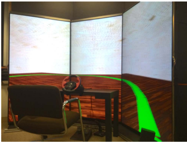
FIGURE 1. The VEHuNT consisted of a cave automatic virtual environment (CAVE) used to present an immersive VR environment to study wayfinding tasks. The VEHuNT consisted of three vertically oriented 4K 80-inch 3D LED screens, with the lateral screens aligned at 45° relative to the central screen. Patients wore polarizing glasses to discern a 3D image during testing and navigated through the virtual environment using a steering wheel and an accelerator pedal.
