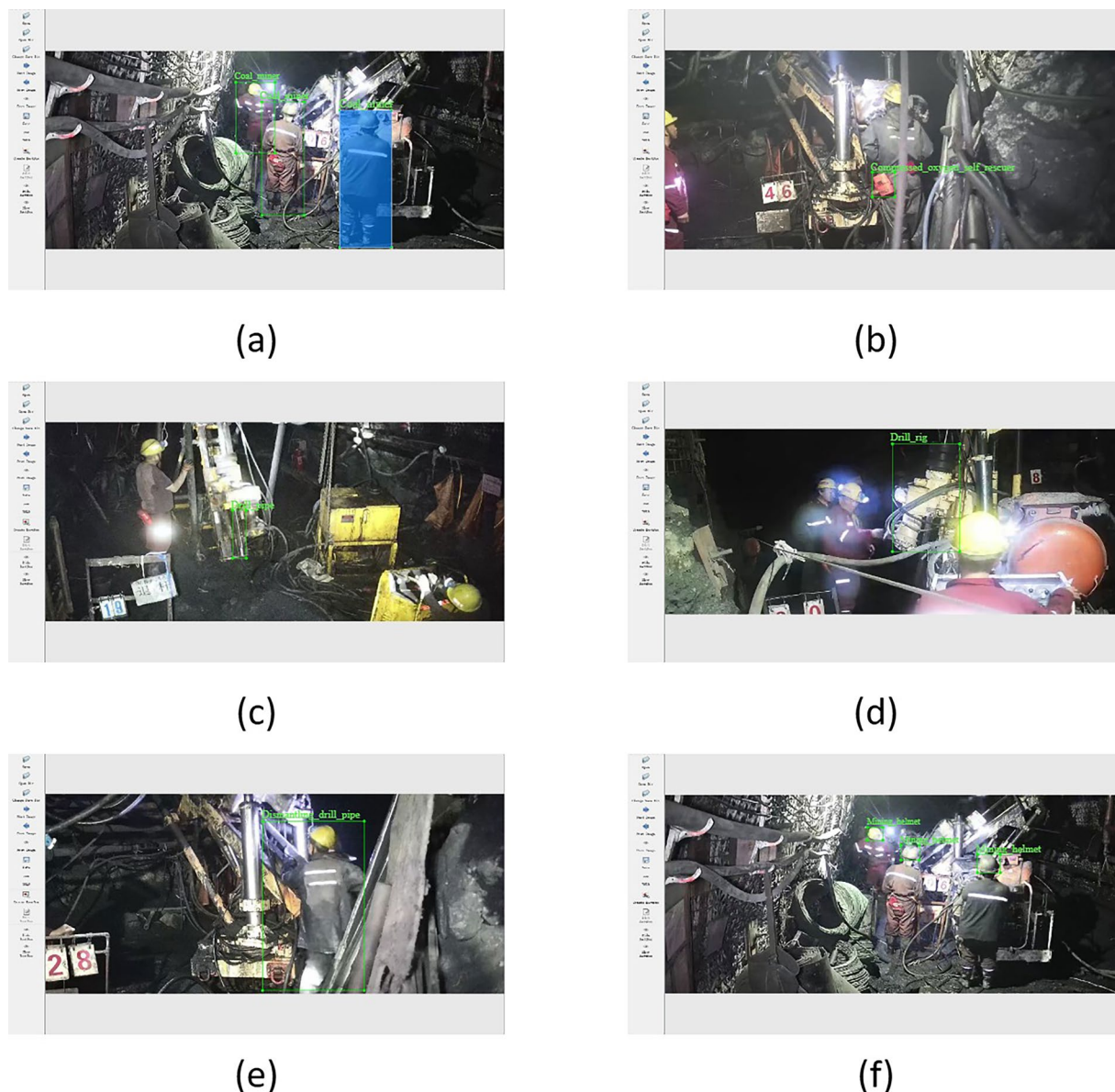
Fig. 4 Annotated labels for the DsDPM 66 dataset: (a) Coal miner; (b) Compressed oxygen self rescuer; (c) Drill pipe; (d) Drill rig; (e) Interaction between miner and drill pipe; (f) Mining helmet.
