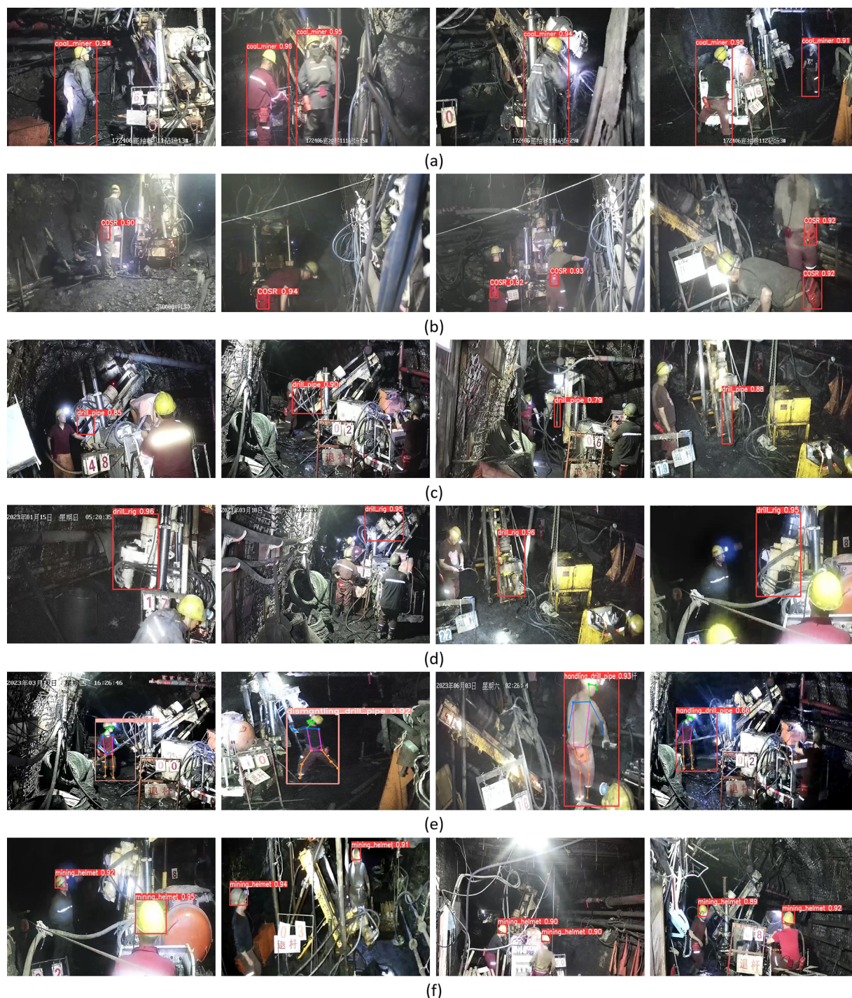
Fig. 7 The validation of the DsDPM 66 datasets by using of the models YOLOv8, Swin-Transformer and DETR. (a) Coal miner; (b) Compressed oxygen self rescuer (COSR); (c) Drill pipe; (d) Drill rig; (e) Interaction between miner and drill pipe and human pose estimation map; (f) Mining helmet.
