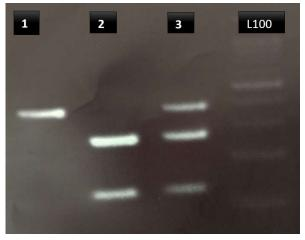
**Figure 2.** Digestion RFLP rs2241880 withe BfuI Enzyme: 1= CC, 386bp - 2= TT, 266bp-120bp - 3= CT, 386bp- 266bp-120bp
