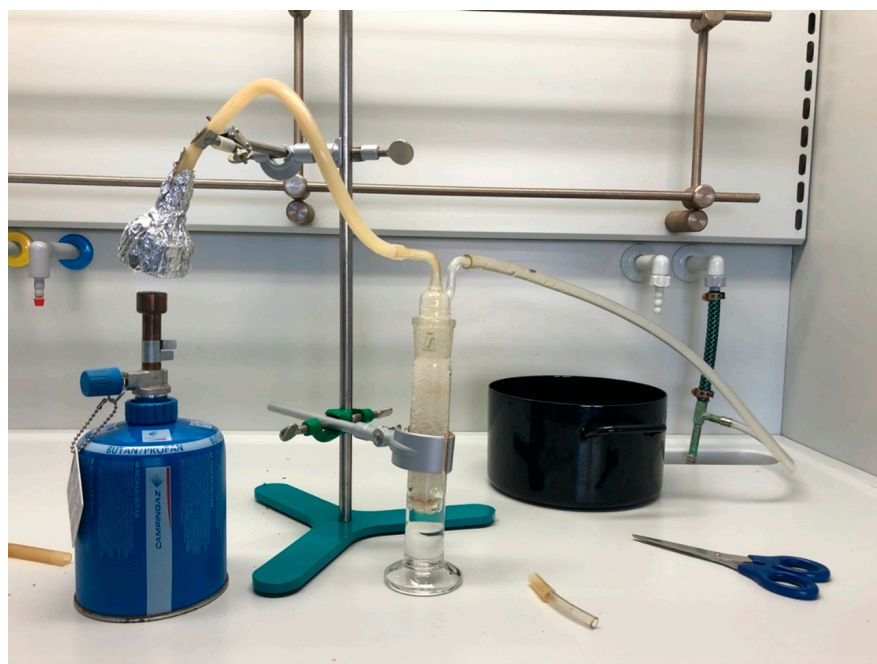
Figure 4. Pipe smoking simulation setup.
