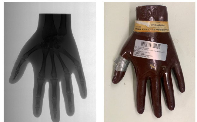
FIGURE 12. Victoreen Nuclear Associate Hand Phantom 76-634 x-ray image taken by SyncBox controlled TDI detector x-ray scanner. 0.5 mm aluminum filtration has been used. Exposure parameters are 60 kVp, 10 mA duration 1.8 sec. Total image acquisition time 5 seconds.
