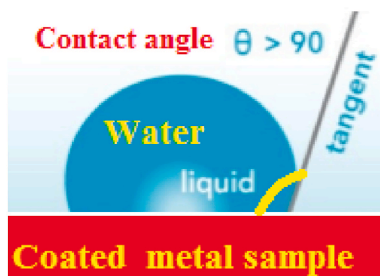
Fig. 4. Schematic representation of measuring contact angle.
