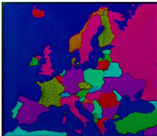
Figure 7. Polarization polychromatic image of femtosecond laser written map of Europe inside fused silica glass. The picture size is 196 \times 167\ \mu\text{m} .
