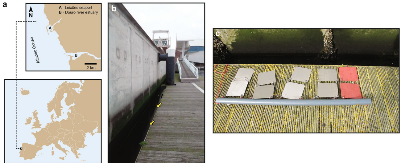
Figure 1. Sampling site: (a) Location of the Cruise Terminal of the Port of Leixões in Northern Portugal, Europe; (b) Marina floating platform; (c) Biofouling monitoring structure composed of ten stainless-steel plates.
