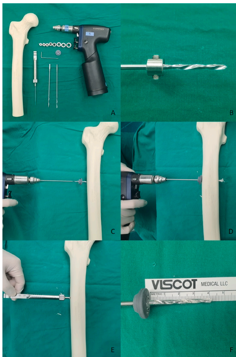
Fig. 2. We provide a step-by-step visual representation of the drilling process. Fig. 2A shows the preparation tools, including the drill with the installed stopper (Fig. 2B). The drilling process is depicted in Fig. 2C and D. After drilling, we measure the bone depth (Fig. 2E) and the total drilling depth (Fig. 2F). The plunging depth is then calculated by subtracting the bone depth from the total drilling depth.
