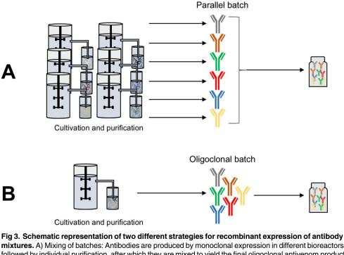
**mixtures.** A) Mixing of batches: Antibodies are produced by monoclonal expression in different bioreactors, followed by individual purification, after which they are mixed to yield the final oligoclonal antivenom product. B) Oligoclonal expression: Antibodies are produced by oligoclonal expression in one bioreactor containing different cell lines. Purification can then be performed on the mix of antibodies, providing the final oligoclonal antivenom.
