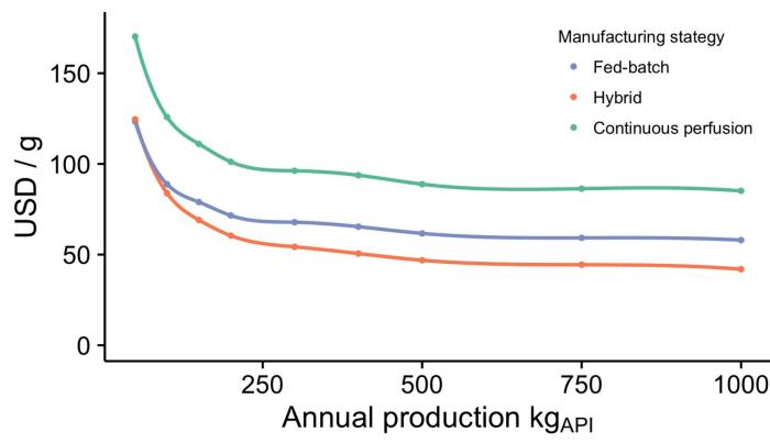
Fig 4. Estimation of Cost of Goods Manufactured (COGM) per gram for oligoclonal antibody production at different scales of production for three different manufacturing strategies, Fed-batch, hybrid, and continuous perfusion (all using chromatography as purification method, see Fig 2), based on cost estimates from [25,31].
