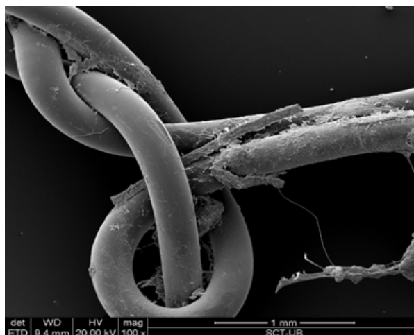
Fig. 4. The Monocryl plus suture knot material seen under the scanning electron microscope, 100x.
