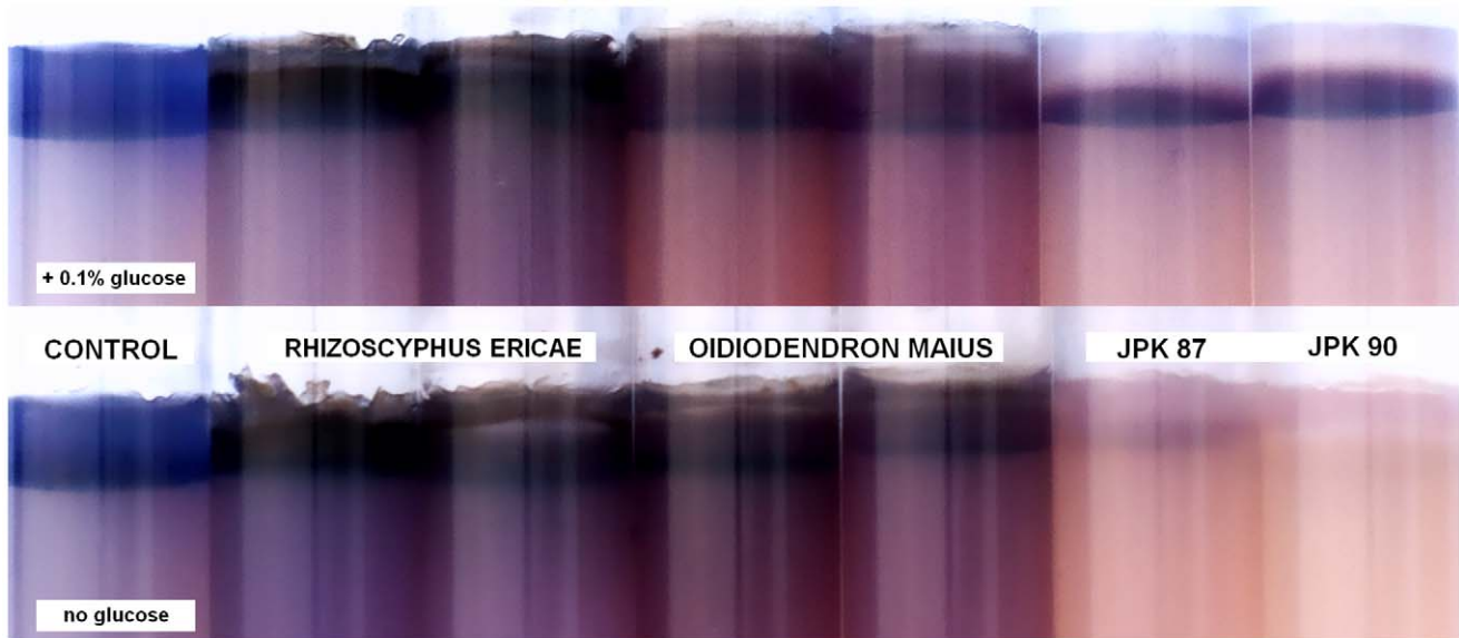
Figure 7. Lignocellulolytic test comparing enzymatic capabilities of ascomycetous ericoid mycorrhizal fungi with the novel basidiomycete. The ability to degrade cellulose azure of representatives of typical ericoid mycorrhizal ascomycetes ( Oidiodendron maius and Rhizoscyphus ericae ) was compared with the basidiomycetous isolates JPK 87 and JPK 90. This test provides a simple, effective assay for both cellulolytic and ligninolytic abilities of the screened fungi; release of azure dye from the upper part of the agar medium indicates cellulose degradation ( O. maius , R. ericae ) while clearing of azure dye indicates activity of ligninolytic enzymes (the basidiomycetes). In the upper row, the agar medium contains 0.1% (w/v) glucose, while glucose is absent in the lower row; it is evident, that the degree of clearing by the basidiomycetes depended on the initial glucose concentration. As complete clearing occurred only on media lacking glucose, we suggest that readily available carbon (e.g., from a host plant) may partly repress ligninolytic activity of the basidiomycetous isolates.
