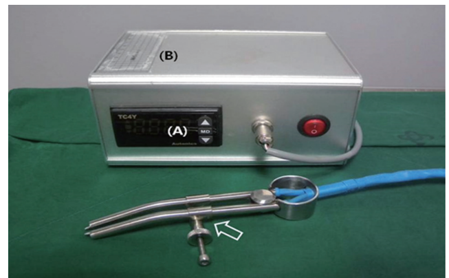
Fig. 1. Modified caliper device. Special compass-like device consisting of temperature display and control buttons (A), scale (B), and thermode with a screw system (arrow).
