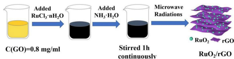
Figure 1. Schematic diagram of RuO 2 nanoparticles anchored on reduced graphene oxide.
