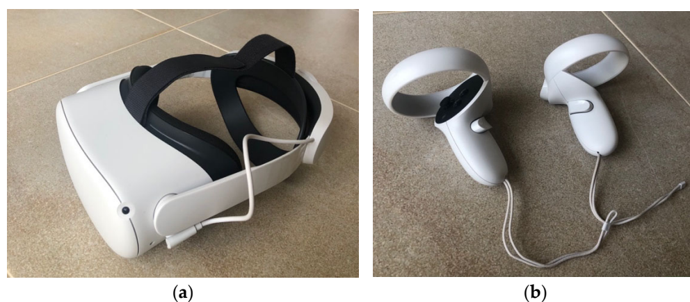
Figure 1. Wearable device used in the study. (a) HMD Oculus Quest 2 + Elite strap and (b) controllers.
