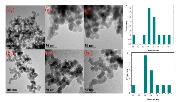
Figure 6. TEM images of (a<sub>1</sub>-a<sub>3</sub>) SNPs, (b<sub>1</sub>-b<sub>3</sub>) SNPs-g-PS and the particle size distribution.
