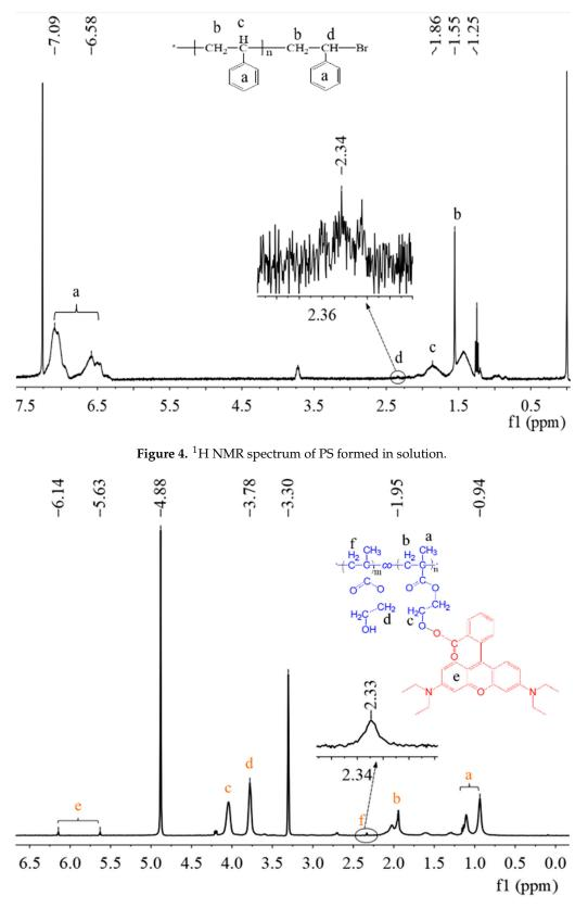
Figure 5. <sup>1</sup>H NMR spectrum of PHEMA-*co*-PHEMA-RhB formed in solution.
