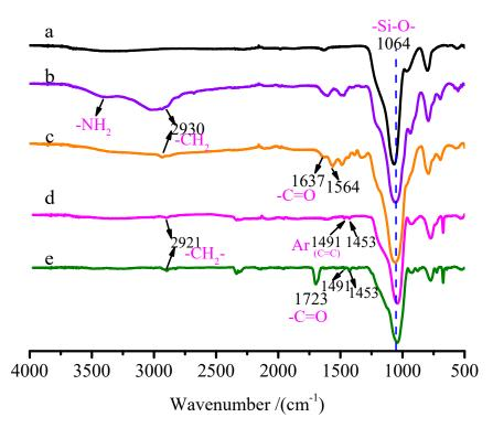
**Figure 2.** FT-IR spectrum of (a) SNPs, (b) SNPs-KH550, (c) SNPs-Br, (d) SNPs-*g*-PS, (e) SNPs-*g*-PS-*b*-PHEMA-*co*-PHEMA-RhB.
