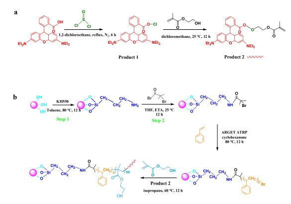
**Figure 1.** General synthetic procedure to fabricate SNPs-*g*-PS-*b*-PHEMA-RhB: (**a**) Synthesis of the HEMA-RhB (Product 2) and (**b**) Synthesis of SNPs-*g*-PS-*b*-PHEMA-RhB via surface-initiated.
