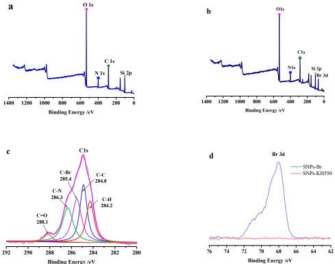
**Figure 3.** XPS spectra of SNPs-KH550 (**a**), and SNPs-Br (**b**–**d**): Survey scan curves range from 0 to 1400 eV (**b**), the C1s core-level spectra (**c**) and Br3d region (**d**).
