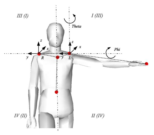
Figure 1. Application of markers on the body landmarks and the corresponding quadrant notation for the left and right arm (Roman numerals in the parentheses are for the right arm). doi:10.1371/journal.pone.0045341.g001
