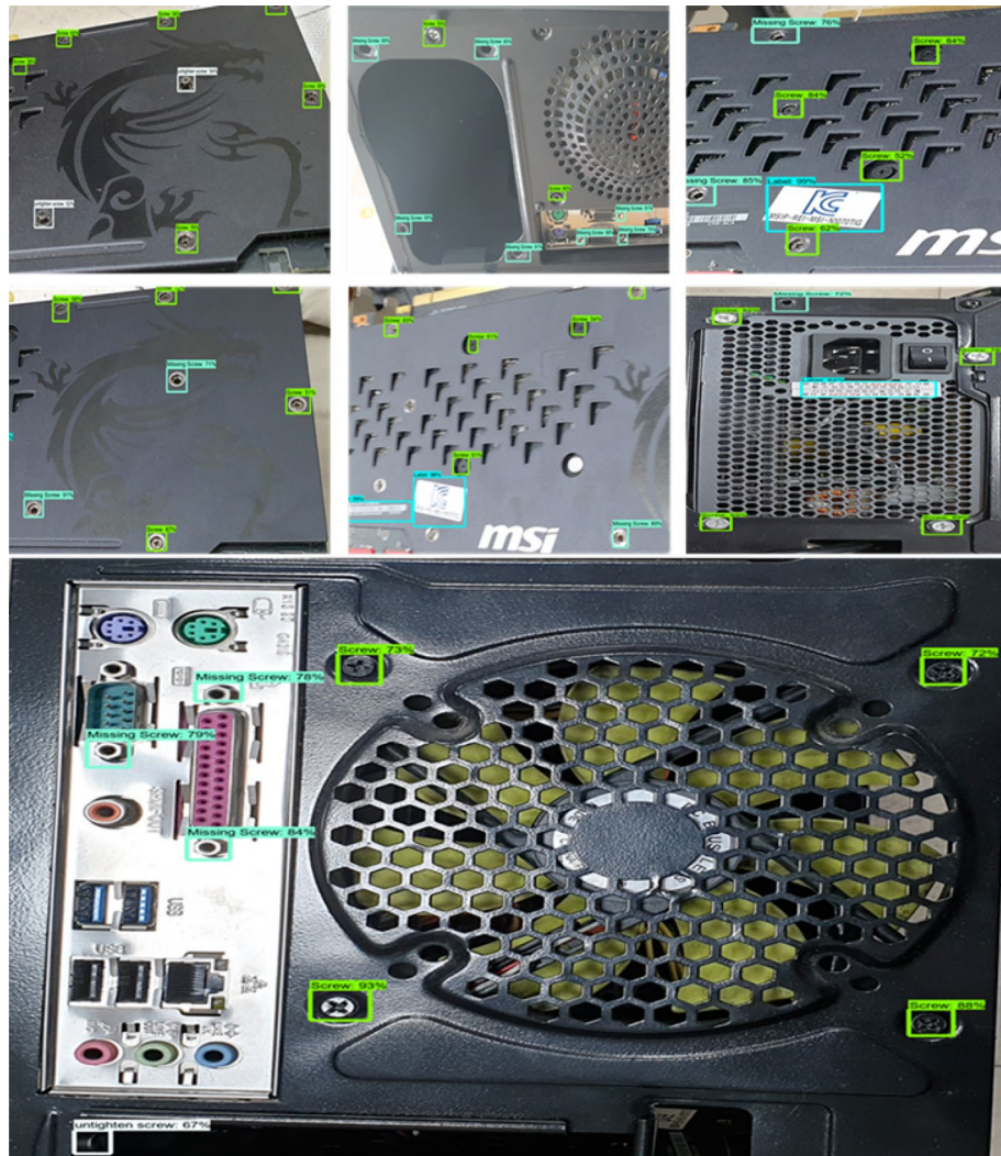
Figure 8. Real-time environmental testing. Model tested on product images, where our four object classes exist, i.e., screws, labels, missing screws, and untight screws.
