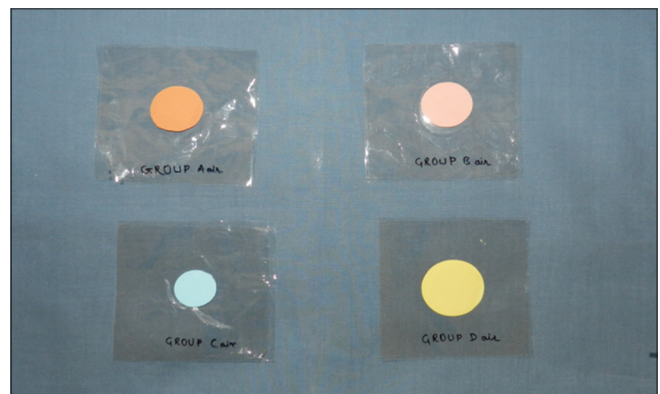
Figure 4: Test samples showing flow of zinc oxide eugenol impression material at room temperature
