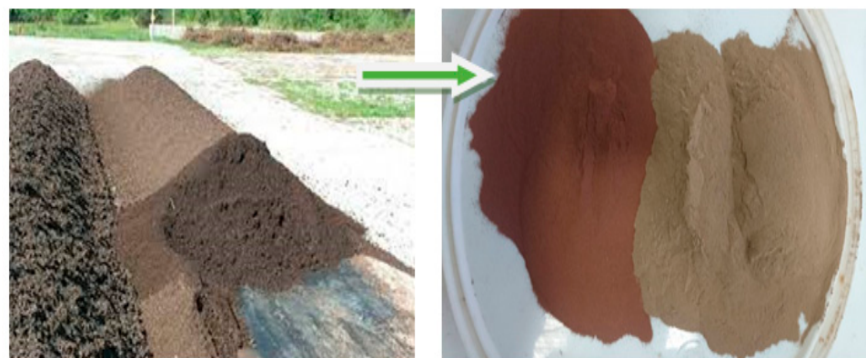
Figure 1. Converted sludge to fly ash from the thermal treatment of sewage sludge—SSA.
