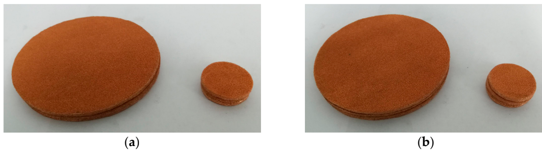
Figure 4. Representative prepared samples for the simple superposed compressed porous metals with the compression ratio of 40%. (a) With the thickness of 9 mm; (b) with the thickness of 12 mm.
