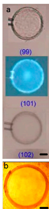
Figure 4. (a) Visualization of the protein rich shell in microgel E during deswelling in 500 mg/L lysozyme solutions (NaCl/tris buffer; pH 8.0, I = 10 mM). Shown are microscopy images taken with without condenser (top), with fluorescent light (middle), and with condenser (bottom) after 99, 102, and 101 min, respectively, after onset of experiment as indicated; scale bar = 25 \mu m. Numbers indicate the time in minutes after exposure to the protein solution; (b) photo of a thin slice through the PSS macrogel with lysozyme-rich shell ( \beta = 0.55 ); scale bar = 2.5 mm.
