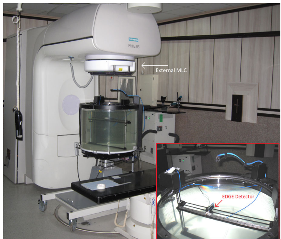
FIG. 3. Equipment used for practical dosimeters, which consist of the SNC 3D Scanner, SNC EDGE detector and the PTW Semiflex ionization chamber.
