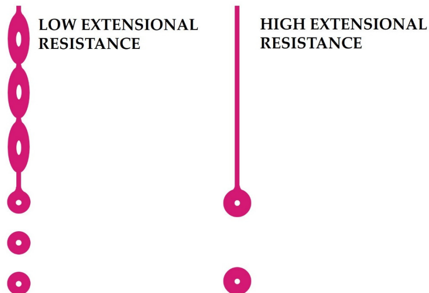
Figure 2. Products with high extensional resistance inhibits droplet pinch-off, tending to result in larger drop sizes. Reprinted from [58].
