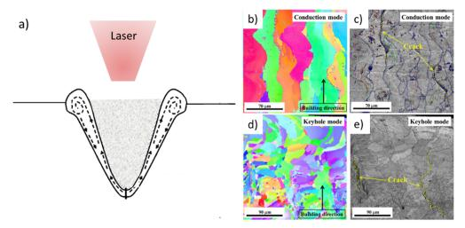
**Figure 6.** (a) Schematic representation of a keyhole melting and EBSD maps of 7050 samples produced in (b,c) a conduction melting mode and (d,e) a keyhole melting mode. (b,d) orientation image map and (c,e) grain boundary misorientation angle map. Adapted from [59], with permission from © 2017 Elsevier.
