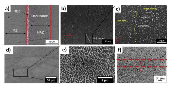
**Figure 9.** SEM images of (a) FVS0812, adapted from [82], with permission from © 2015 Cambridge University Press; (b,c) Al-Si-Ni-Fe water quenched and aged at 250 °C for 5 h, adapted from [83], with permission from © 2019 Elsevier; (d,e) Al-Si-Ni, adapted from [33], with permission from © 2017 Elsevier; and (f) Al-20Si-Fe-Cu-Mg adapted from [68], with permission from © 2016 Elsevier.
