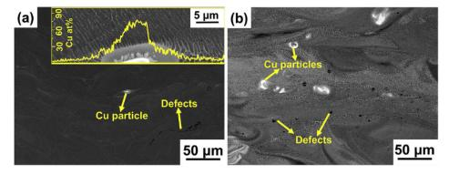
**Figure 4.** Backscattered Electrons (BSE) SEM micrographs of LBF (a) Al-6Cu and (b) Al-40Cu alloy (inset: Cu distribution across the Cu-rich zone), adapted from [38], with permission from © 2018 Elsevier.
