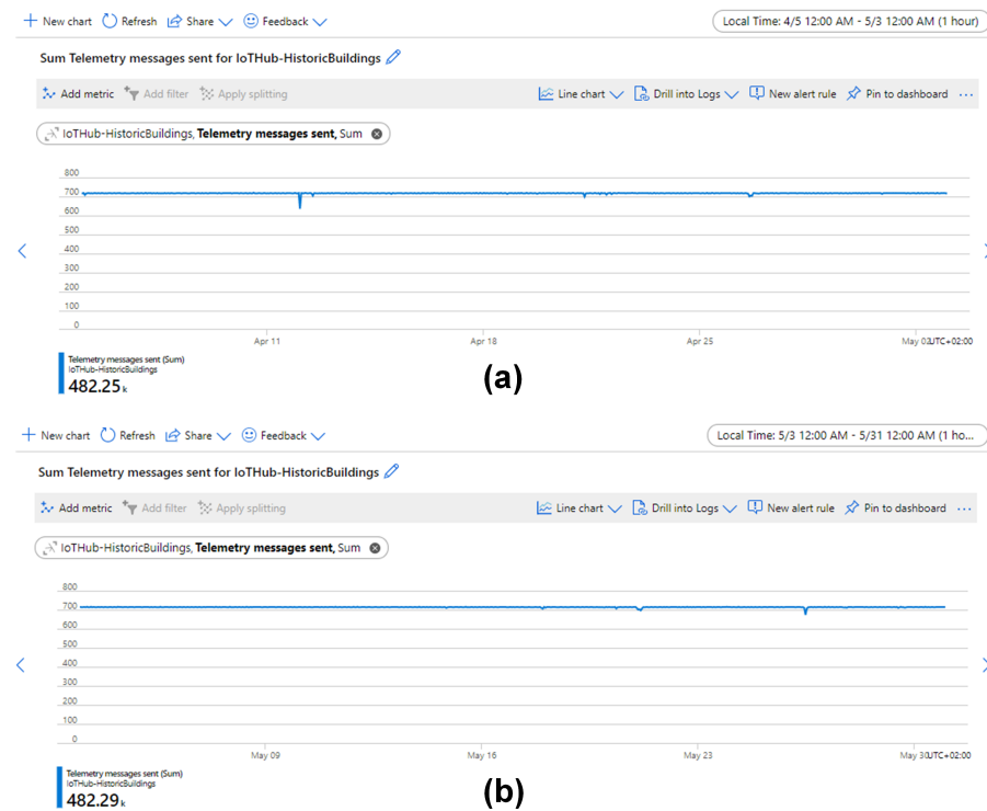
Figure 12. Hourly aggregated metrics for messages sent from edge to IoT Hub between 5 April and 31 May. The total number of sent messages was \sim 964,540 . Among them, (a) \sim 482,250 messages were sent between 5 April and 3 May and (b) \sim 482,290 messages were sent between 3 May and 31 May.
