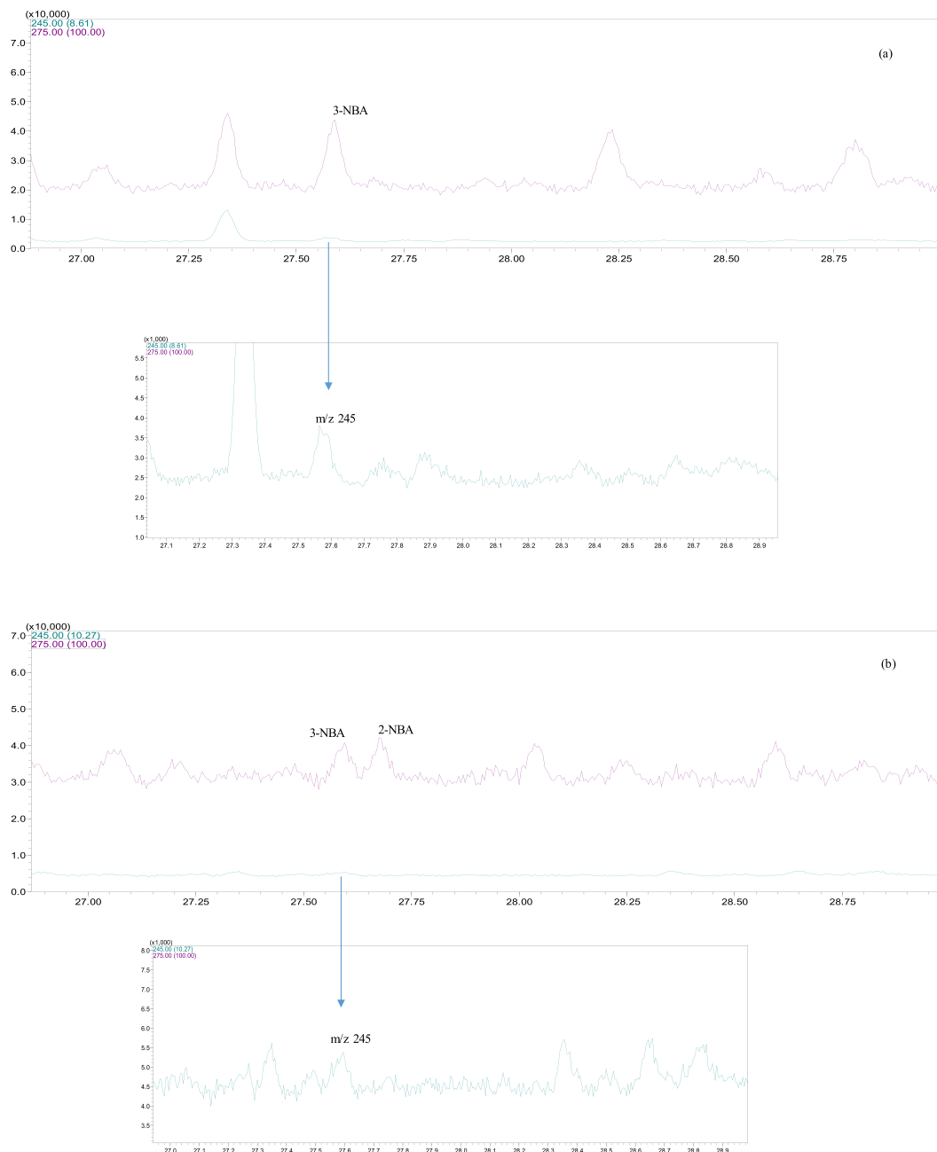
Figure 1. Chromatograms of 3-NBA and 2-NBA. (a) Bus station real PM sample, (b) ambient particulate sample from the coastal site. Limits of detection are 2.0 pg and 2.4 pg for 2-NBA and 3-NBA, respectively.
