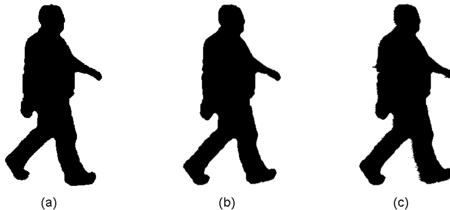
FIGURE 5. (a) Originally extracted silhouette, (b) rotated silhouette, (c) rotated silhouette with added emerging points.
