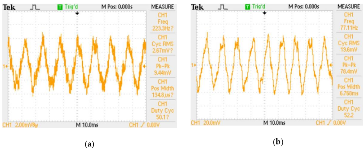
Figure 5. Waveforms at output of flow transducer: (a) Signal straight from output of flow transducer; vertical sensitivity in oscilloscope channel 2 mV/division; (b) Signal after amplification by active differential probe; vertical sensitivity in oscilloscope channel 20 mV/division.
