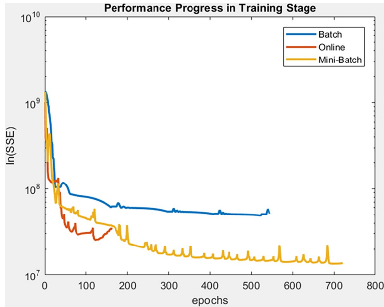
Fig 25. Performance progress of SEE in training stage by learning method to engine behavior dataset.
