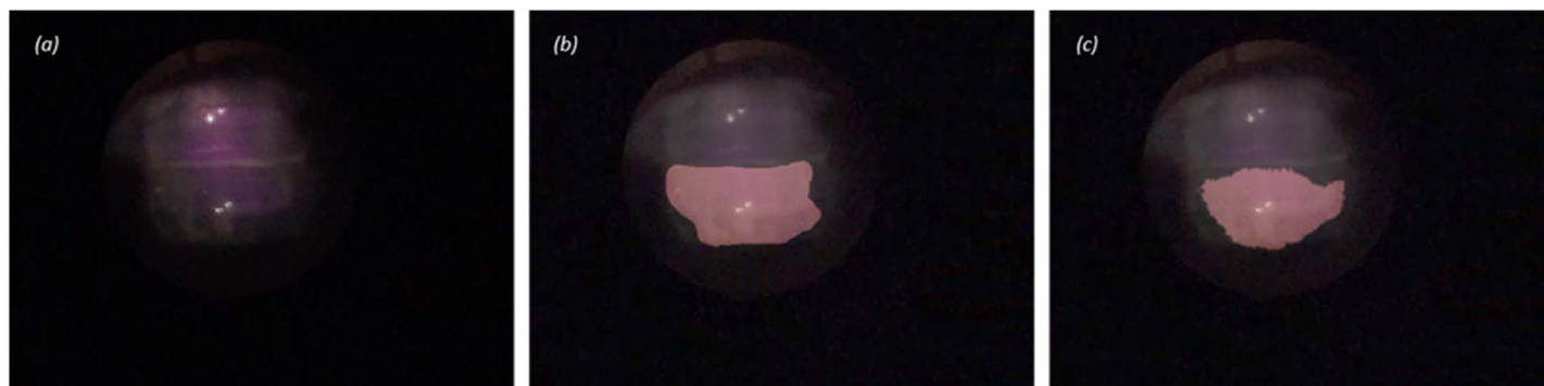
Fig 6. Sample dual perfusion chamber (top and bottom) image (a), manually generated bottom chamber outline overlayed on original image (b), AI generated bottom chamber outline overlayed on original image (c).
