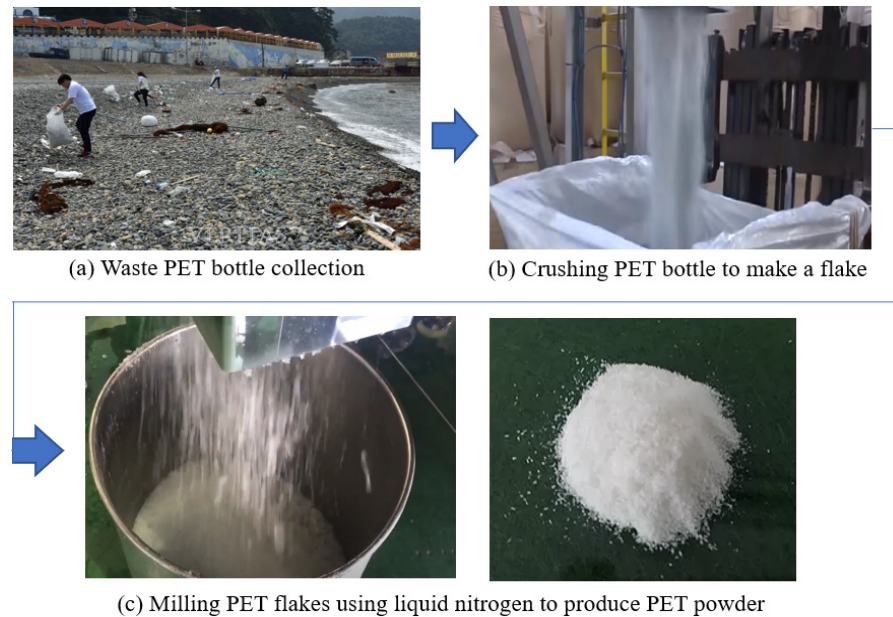
Figure 1. Preparation process of PET powder. (a) Waste PET bottle collection; (b) crushing PET bottle to make a flake; (c) Milling PET flakes using liquid nitrogen to produce PET powder.
