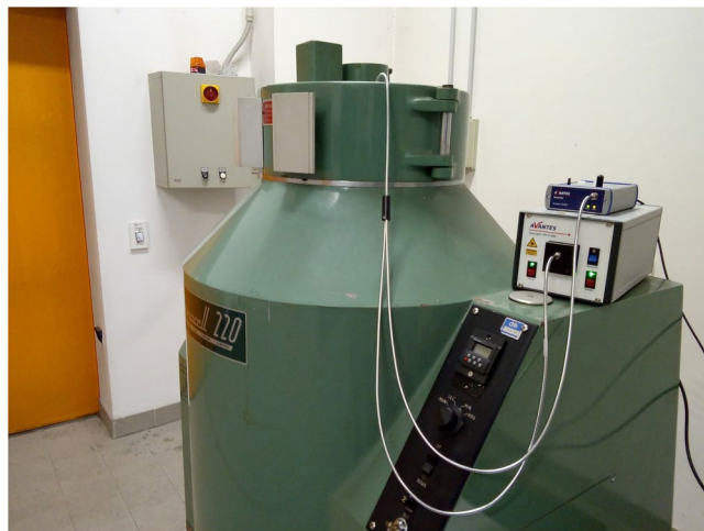
Figure 6. Picture of the Gammacell220 of ISOF-CNR at Bologna. During the operation the optical fiber probe is inside the irradiator. The light source and the spectrometer are remotely controlled.
