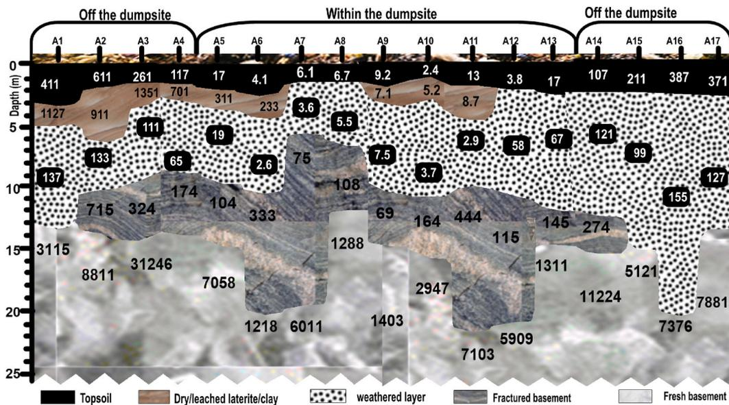
Fig. 3. Geoelectric/geologic profiles of the dumpsite showing the resistivity values along West – East azimuth. The resistivity values is a reflection of the dumpsite leachate infiltration of the subsoil.
