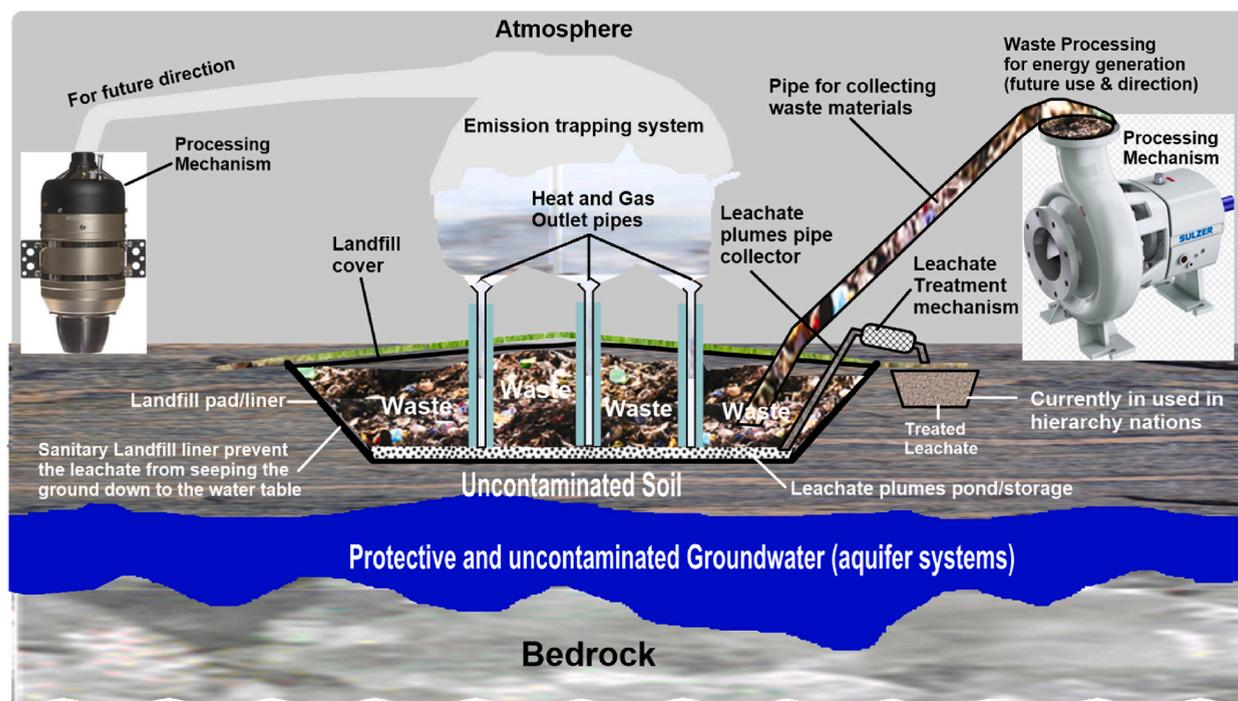
Fig. 10. Proposed modern sanitary landfills for future direction with modern technologies for total environmental security and sustainability.
