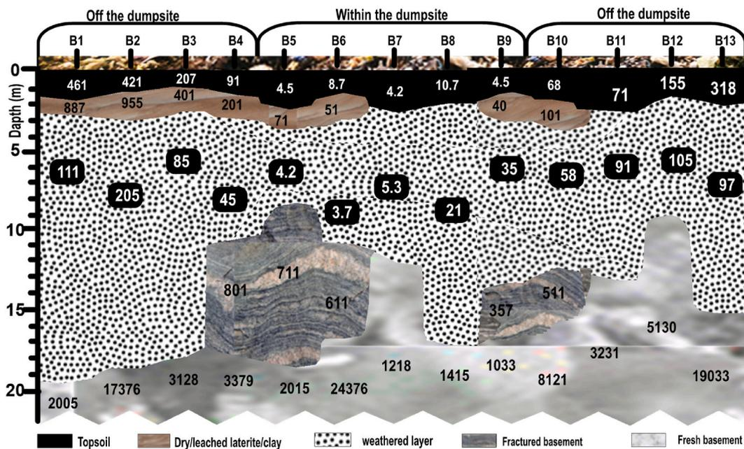
Fig. 4. Goelectric/geologic profiles of the dumpsite showing the resistivity values along North – South azimuth. The resistivity values is a reflection of the dumpsite leachate infiltration of the subsoil.
