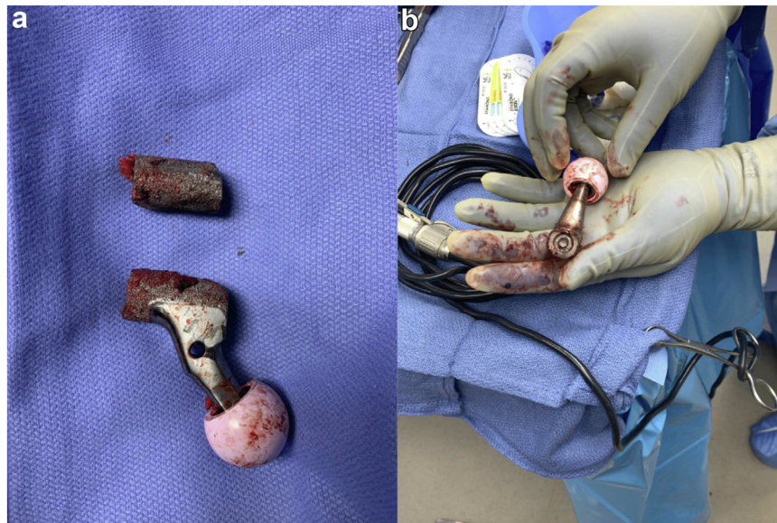
Figure 5. (a) Intraoperative photograph demonstrating proximal body fracture of the Arcos revision femoral stem following explantation, (b) without evidence of corrosion at the head-stem trunnion.
