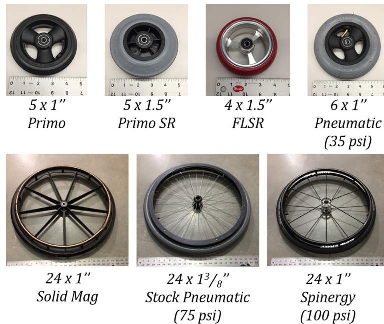
Fig 5. Tested components. Array of components representing a range from standard, off-the-shelf wheelchair configurations to costlier up-charged versions.
