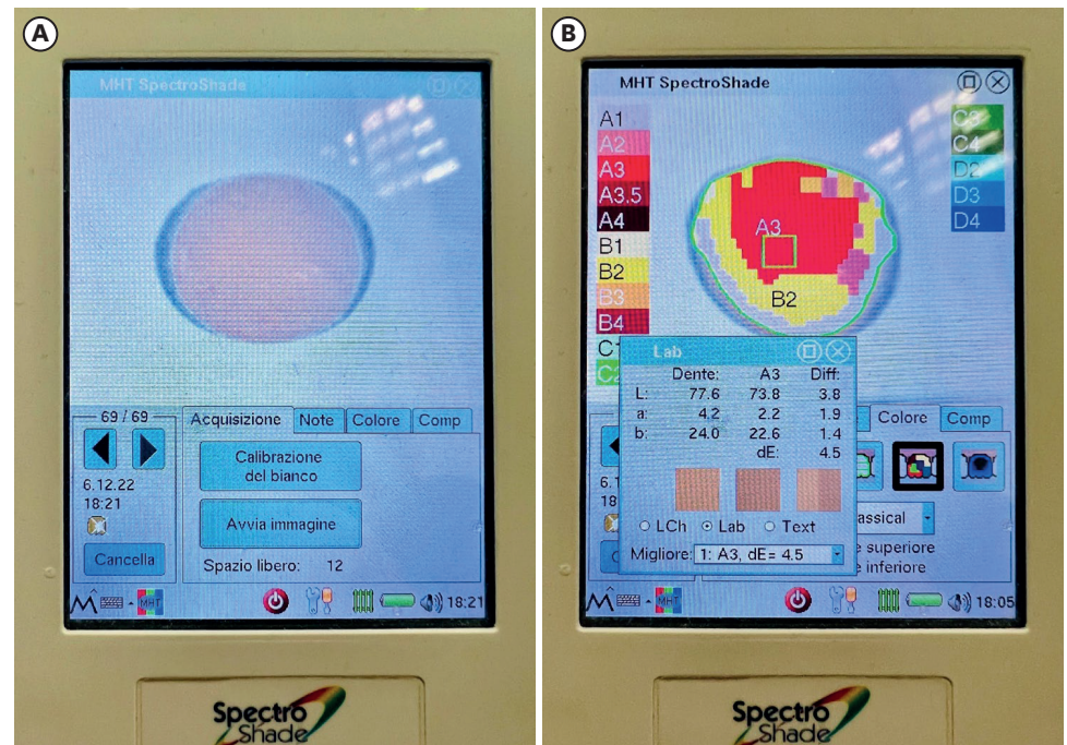
Figure 1. Procedure for using spectrophotometer on composite samples. A sample before (A) and during (B) the spectrophotometer measurement, the spectrophotometer was used to measure the CIE L^* a^* b^* color parameters.
