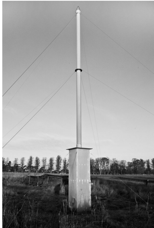
Fig. 1. A suction-trap that samples migrating insects at a height of 12.2 m. The vertical 9.2-m pipe has an internal diameter of 244 mm. The 3-m housing at the base of the trap contains a motor and an electric fan from which a sample volume of 0.75 m 3 air per second is generated. Aphids and other insects flying over the trap are pulled down through the vertical pipe into a collecting bottle inside the housing.
