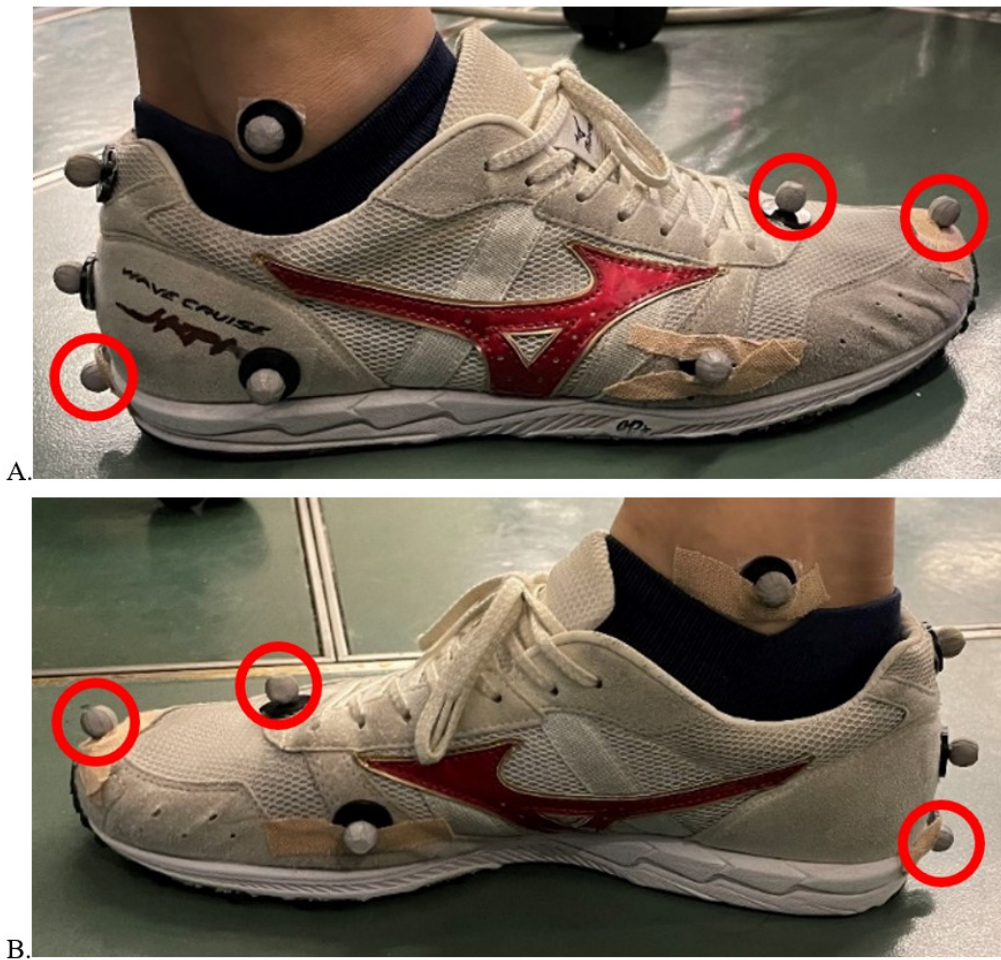
Figure 1. Ten reflective markers (three tracking markers with red boundaries and seven anatomical markers) on the right shoes of the participant: A. lateral view and B. medial view.
