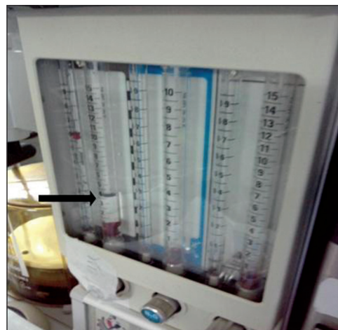
Figure 1: Arrow showing influx of water in air flowmeter
