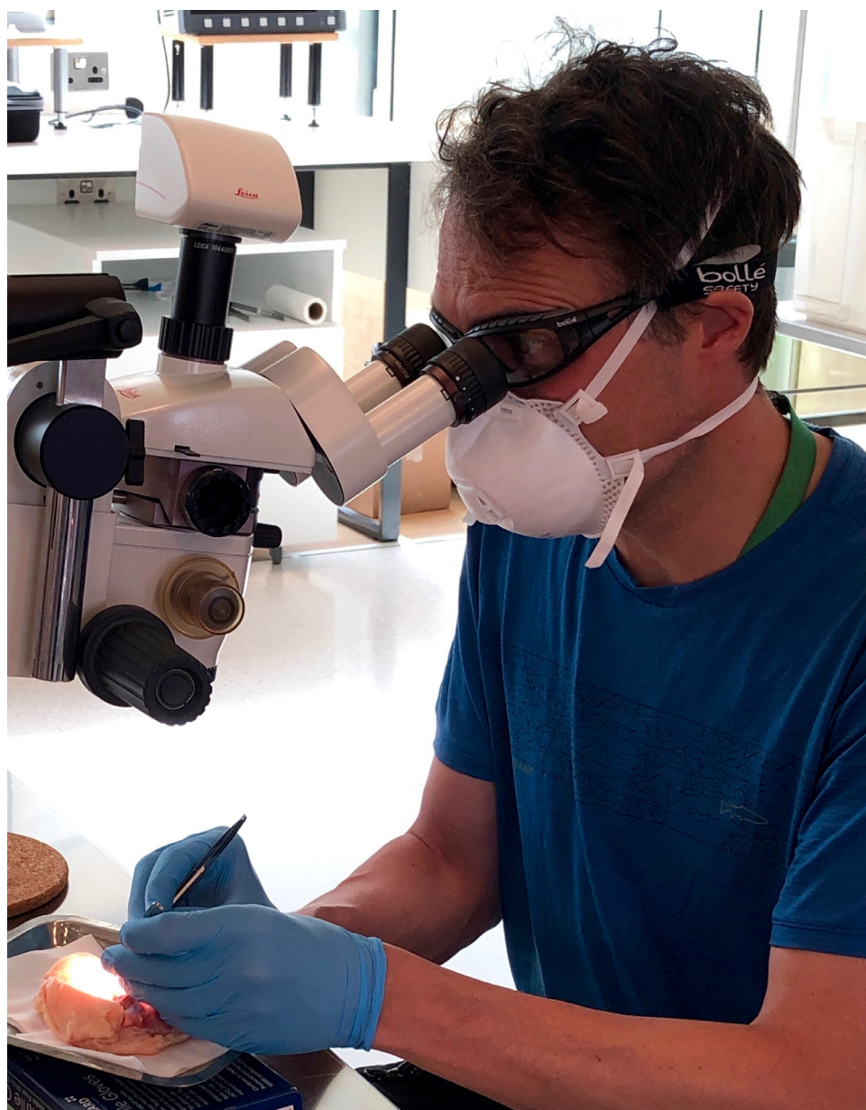
Figure 1 The combination of FFP3 respirator and elasticated sports goggles was compatible with the operating microscope, when trialled in the surgical skills lab.
